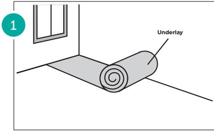
Place the underlay (foam) on the floor and check what tongue & groove profiles are.
