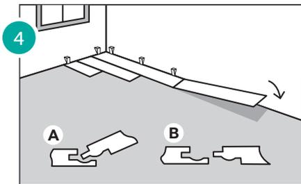
Connect the short side tongue click to the groove click at a 30-degree angle, aligning them on the floor as shown in figures 4A and 4B. Ensure that the click sides face the wall. Next, trim 1/3 of another laminate panel and connect it adjacent to the 2/3 of the previous panel, with the cut side facing the wall.
