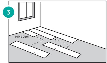
Place a whole panel whose tongue sides of laminate flooring face the corner. After that cut 2/3 of another panel and connect it to the whole panel whose tongue click sides face to the wall. After that cut 1/3 of another laminate flooring, connect it next to the 2/3 of laminate flooring. So cut side of the 2/3, 1/3 of the panel face to wall.
