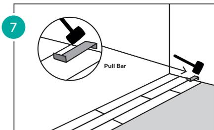
Laminate flooring is fixed by hammering with pull bar and tapping block.
