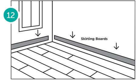
Skirting boards are cut depending on how they fit to be ready for installation. Fix the skirting boards to the walls, using a hammer and nails.
