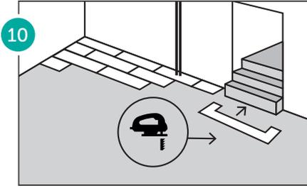
Laminate flooring is cut on the sides by having minimum 15mm gap according to stair step and fit them appropriately.
