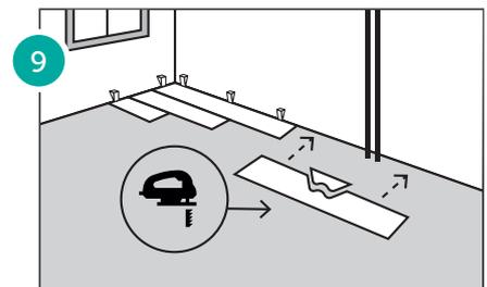
During installation, cut sections of the panels facing heating pipes with a 15mm gap using appropriate cutting tools. Glue the cut pieces together with adhesive, ensuring click sides face the wall. Then, trim 1/3 of another laminate flooring and connect it beside the 2/3 piece, ensuring the cut side faces the wall.
