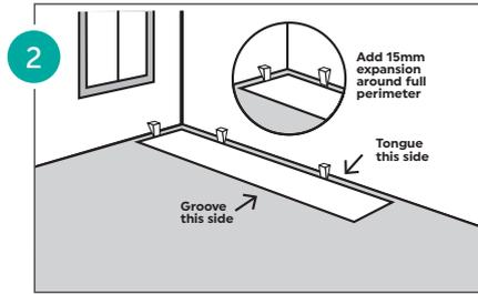
Start installation with the first line from the left corner of the room by meeting both tongue click sides of the panel to the wall. While starting the installation, place the distance protector (wedge of 15mm thickness) that ensures distance with the wall.
