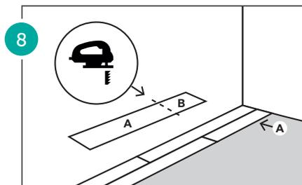
By calculating the distance of wedge laminate flooring is marked as A and B, then it is cut and click on the long side of panel is get connected. If the part B is longer than 30cm, it can be used at the beginning of the next line. 8.
