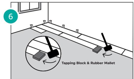
Push to the tapping block by rubber mallet on the short side of the panel to lock the clicks. Not to damage the clicks on the panels avoid hard impact.
